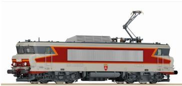
The BB 15000 is an electric locomotive class of the National French Railways (SNCF) for use on the AC 25 kV 50
